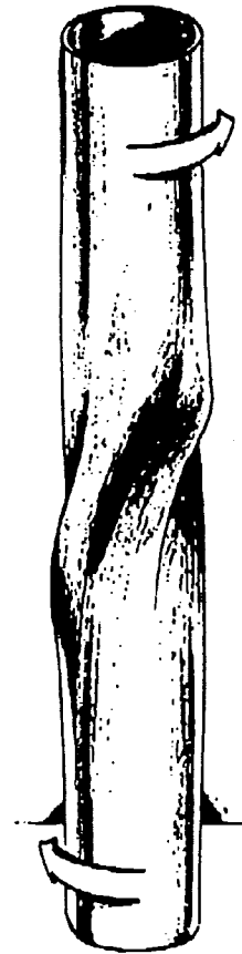
Figure D-6. Torsion load failure
