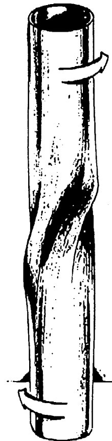
Figure D-6. Torsion load failure
